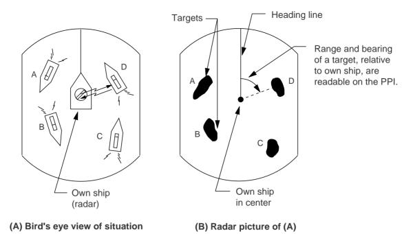
Figure 1-1 How radar works
